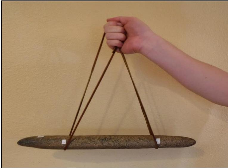
Figure 3. Suspending a potential lithophone for testing horizontally. It is suspended by thin pieces of leather on the two acoustical nodes (dull zones) marked with white tape.
