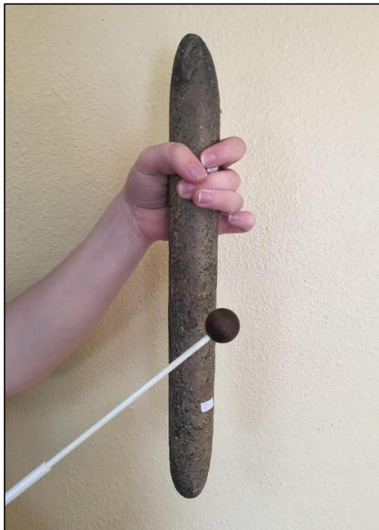
Figure 2. Testing a potential lithophone vertically by holding it at the point of the upper acoustical node (dull zone). The least amount of contact with the hand/fingers provides the most resonance.
